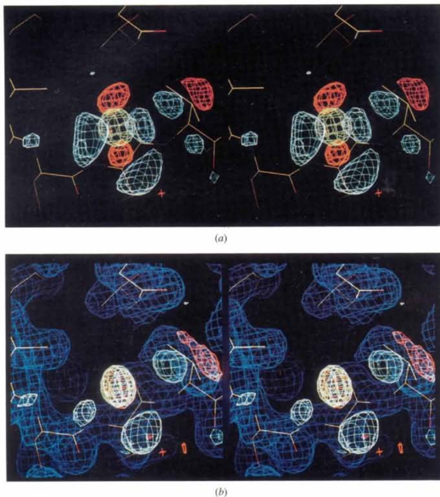
Fig. 9. Residual maps after heavy-atom parameter refinement with the program SHARP (stereoviews). (a) The heavy-atom parameter refinement used an isotropic thermal factor for the Kr atom. Displayed are the current heavy-atom model (in green – a single isotropic Kr atom) and the isomorphous residual map (red for positive density, light blue for negative density). This map is based on the gradient of the log-likelihood function and indicates discrepancies between the current heavy-atom model and the experimental data. The two pairs of positive and negative residual density peaks that are situated in orthogonal directions relative to each other around the heavy atom strongly suggest anisotropic thermal movement of the krypton atom. (b) The heavy-atom parameter refinement used an anisotropic thermal factor for the Kr atom. The positive and negative density peaks around the heavy atom are no longer present. The residual map only shows two negative peaks close to the krypton site (towards the bottom of the figure) that could correspond to replaced water molecules as well as a pair of positive and negative density peaks (near the side chain of Val209) that could correspond to a side-chain displacement. Also displayed (in yellow) is a standard difference-Fourier map computed with terms |F_{\text{derivative}}| - |F_{\text{native}}| as amplitudes and phases calculated from the refined native structure. This difference-Fourier map displays a peak at the krypton binding site whose shape is in perfect agreement with the current heavy-atom model (in green), thus validating the use of an anisotropic thermal parameter refinement. The final SIRAS electron-density map after density modification is shown in blue. Superimposed to these maps is the refined native structure of the PPE molecule.
